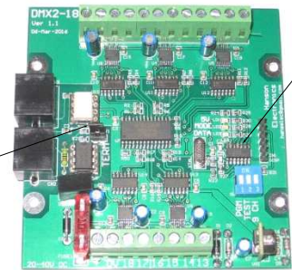
Start address set via dipswitches
