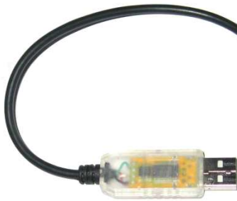
USB dongle connects to PC, Pi or BBB
