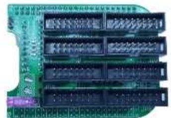
Same as the RTC version but with shorter header pins and no clock module under the P10 connectors.
